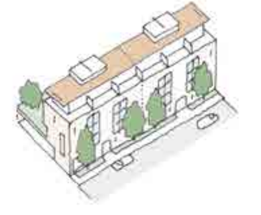
Typology: Stacked maisonettes / flats Density: Medium - High Parking: On-street, parallel arrangement integrated into street design Where: Village centre
