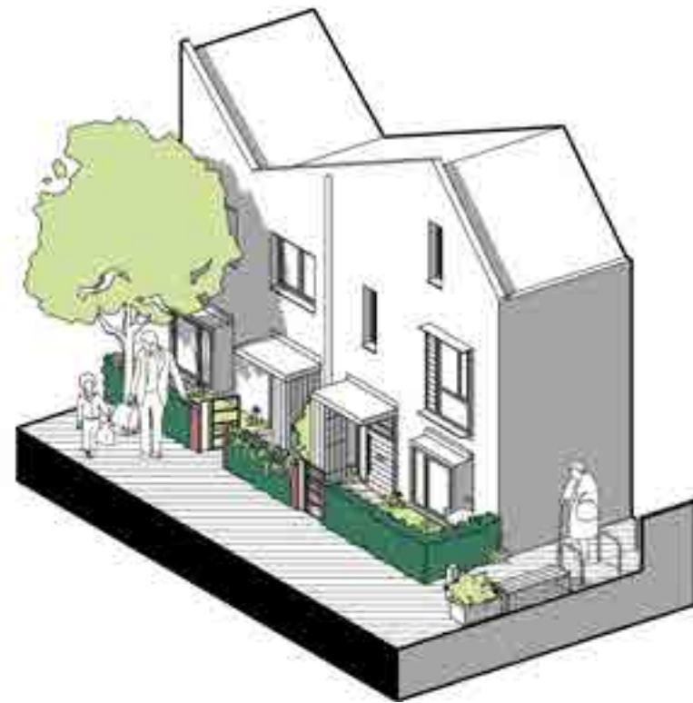
A shallow front garden threshold defined by a low wall boundary treatment, creating a strong relationship between the building and the street
