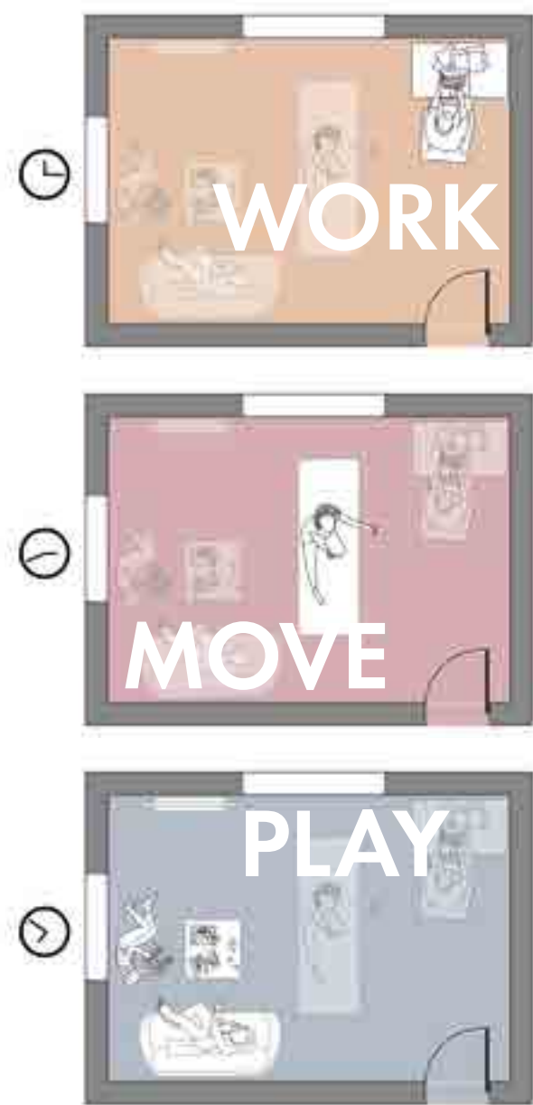
Flexible internal layouts allow rooms to be multifunctional and minimise conflict between space demands
